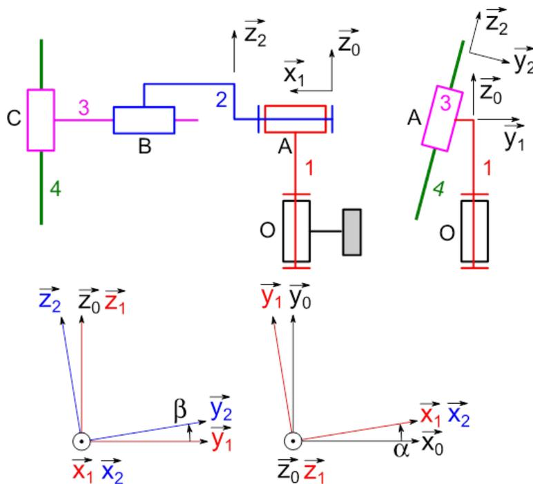
$$\overrightarrow{OA} = H\vec{z}_0 - e\vec{y}_1 \quad \overrightarrow{OG_1} = h_1\vec{z}_0 \quad \overrightarrow{AB} = L\vec{x}_1 \quad \text{avec } L = 65 \text{ cm et } e = 10 \text{ cm}$$
