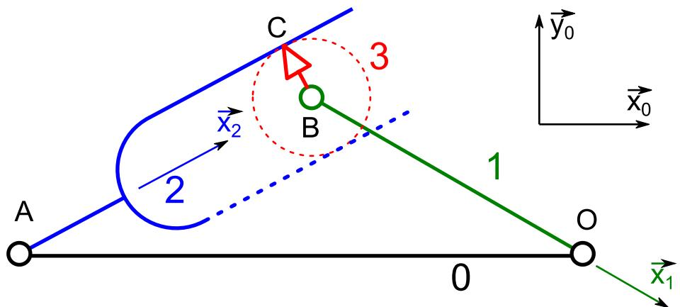
$$\overrightarrow{AB} = X(t) \cdot \vec{x}_2 \quad \theta = (\vec{x}_1, \vec{x}_2) \quad \alpha = (\vec{x}_2, \vec{x}_0) \quad \tan \alpha = \frac{\sin(\theta)}{\cos(\theta) - \sqrt{2}} \quad X(t) = R \cdot \sqrt{3 - 2\sqrt{2} \cdot \cos(\theta)}$$
