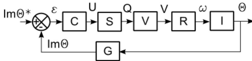
$$S(p) = \frac{K_s}{1 + \frac{2\xi_s}{\omega_{0s}}p + \frac{1}{\omega_{0s}^2}p^2} \quad V(p) = \frac{K_v}{1 + \frac{2\xi_v}{\omega_{0v}}p + \frac{1}{\omega_{0v}^2}p^2} \quad G(p) = \frac{1}{\pi/2} = \frac{2}{\pi}$$
